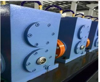
> 4.1.4. Horizontal roll frame & Vertical roll frame
